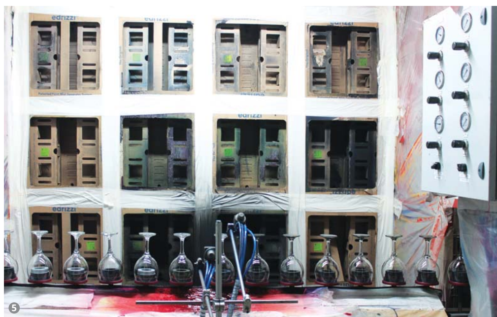
Figure 5: The line is equipped with dry filtration systems with the Edrizzi® technology.
