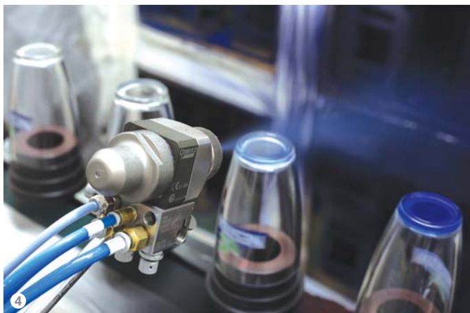
Figure 4: The automatic application of liquid coatings provided by Pinturas Benicarlò (Grupo Ferro SL).
