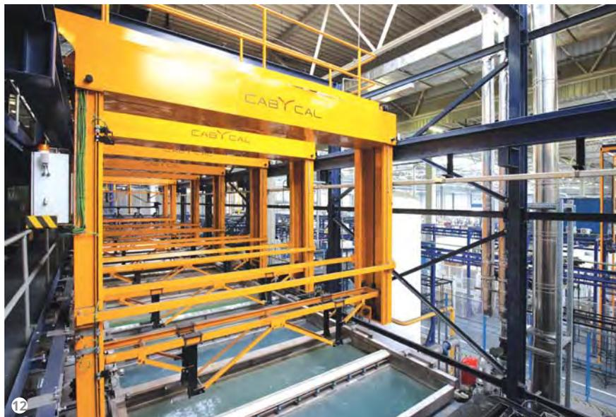
Figure 12: The cataphoresis line is equipped with 8 bridge cranes.
