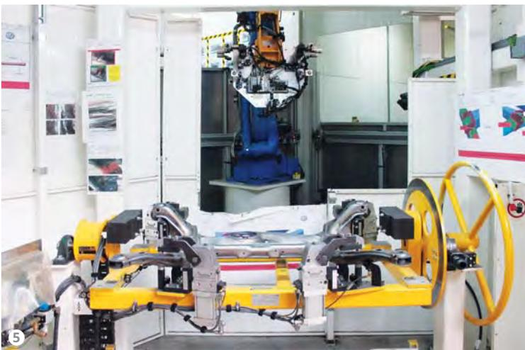
Figure 5: The robot that picks up the chassis from the line.
