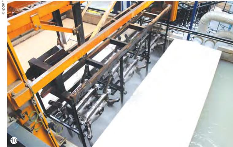
Figure 10: The spray cleaning tank.
