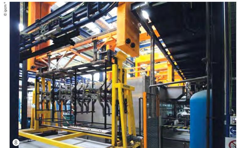
“Gestamp needed to relieve the operators from the loading and unloading of the chassis, the heaviest components produced, by automating them. Cabycal solved the problem by integrating a two-rail conveyor that splits in two handling lines: a manual one for the loading of the smallest and lightest parts on hanging frames and a fully automated one featuring two robots and elevators.”
