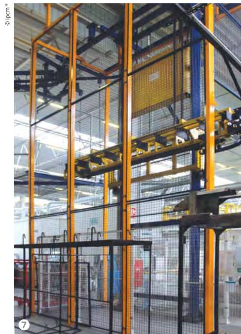
Figure 7: The elevator that takes the cages to the overhead storage buffer.
