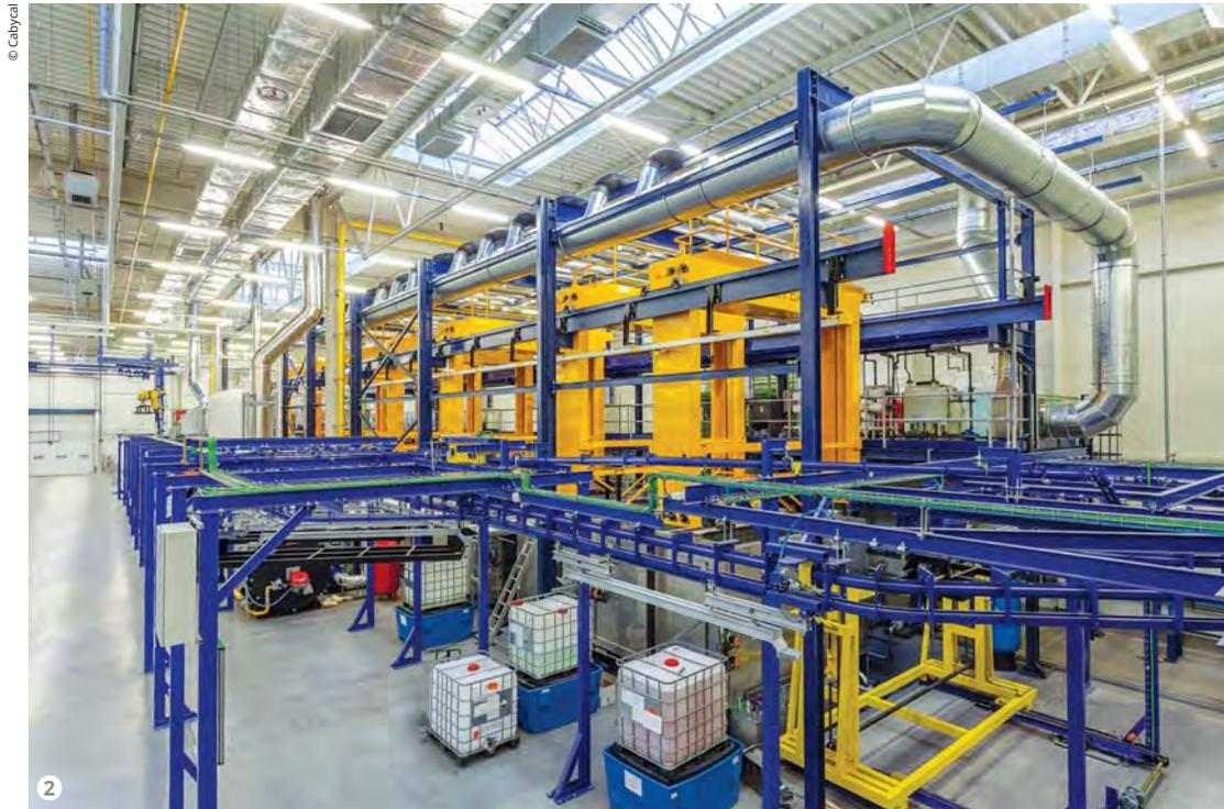
Figure 2: The cataphoresis plant supplied by Cabycal.
