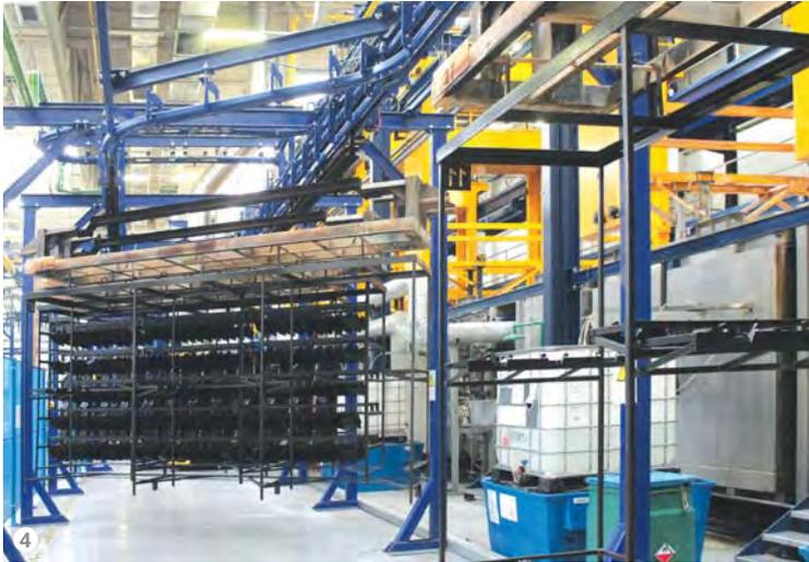
Figure 4: The manual handling line devoted to small and light workpieces.
