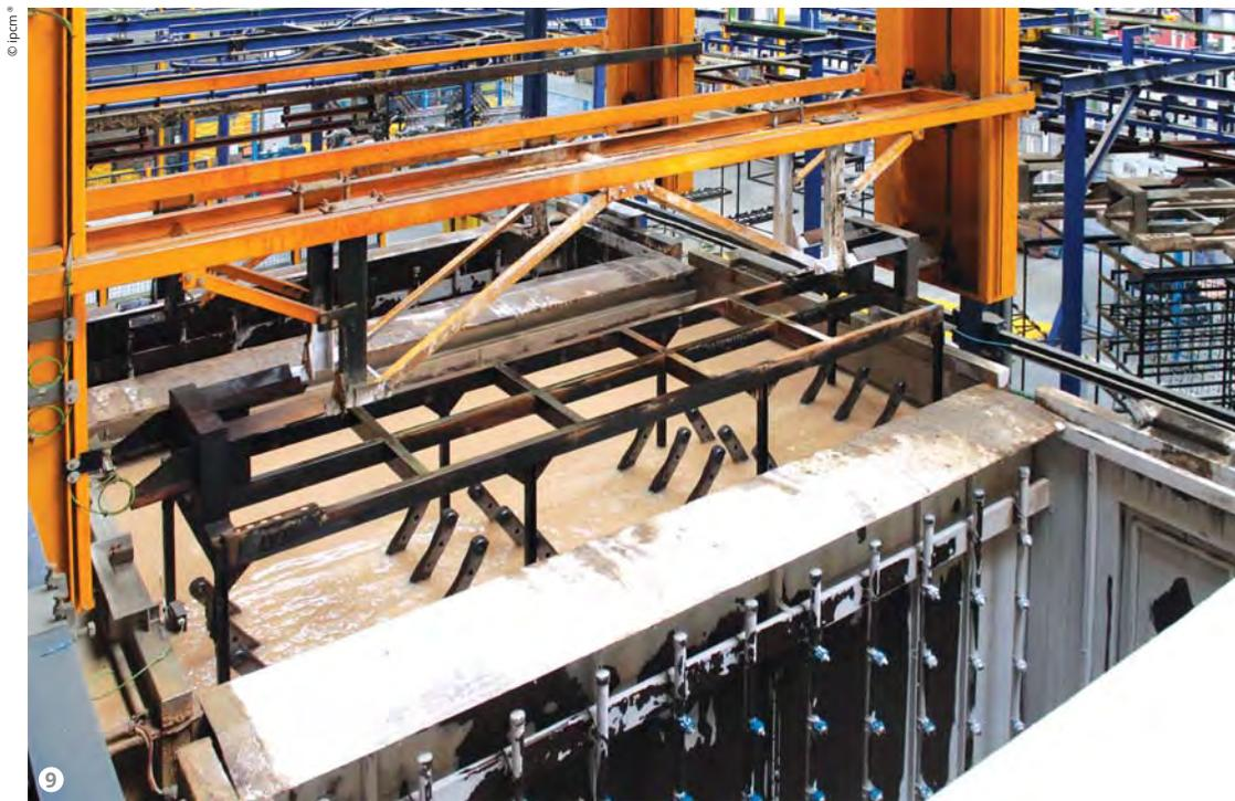
Figure 9: The hot immersion degreasing tank.
